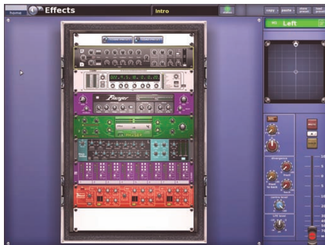
Typical Effects screen containing all of the available effects. (The PRO3 only has six rack unit positions.)
