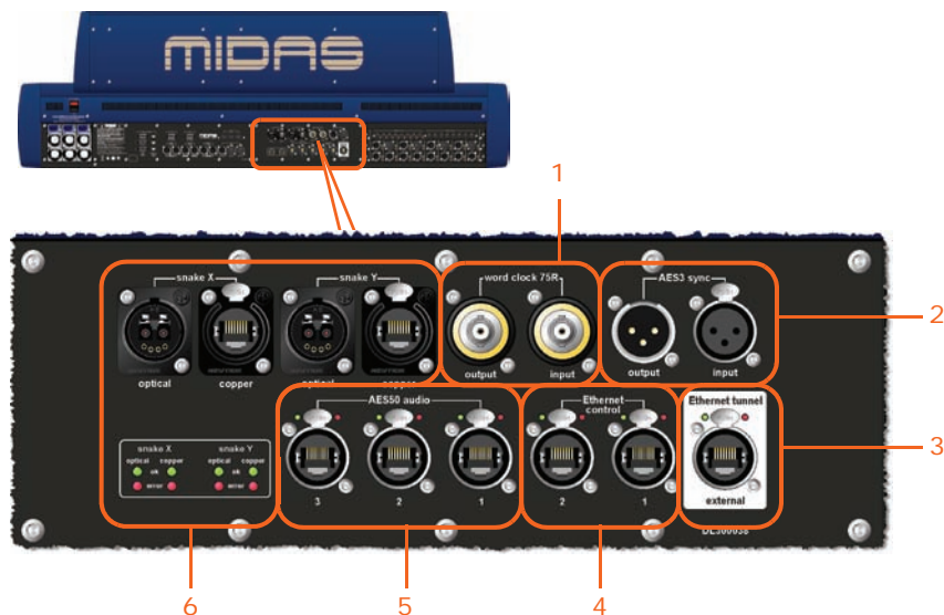
Typical audio, networking and synchronisation connections on the rear panel of a PRO Series Control Centre
