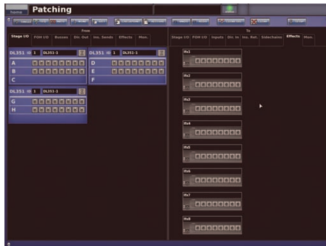
Patching screen showing the location of the effects in the Effects tab of the To section. (PRO3 only has a maximum of six effects.)
