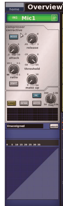
Compressor processing area
