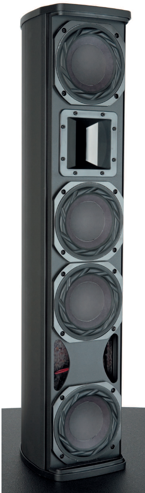
2 1/2-way box comprising a line source of frequency-dependent length for the low midrange combined with a 90° x 40° horn
