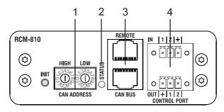
Illustration 4.1: Controls and Connections of the RCM-810
