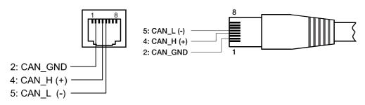
Illustration 4.2: Pin-assignment of CAN jack and CAN plug
