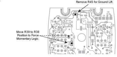
Figure 3: PCB Jumper Locations
